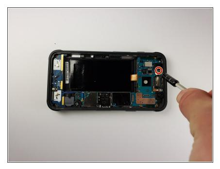
Use a Phillips 000 screwdriver to remove the screw covering the proximity sensor.
