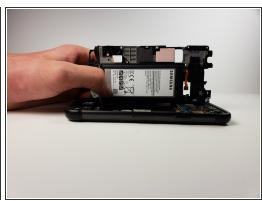
Use a metal spudger to pull the mid frame and battery off of the motherboard.
