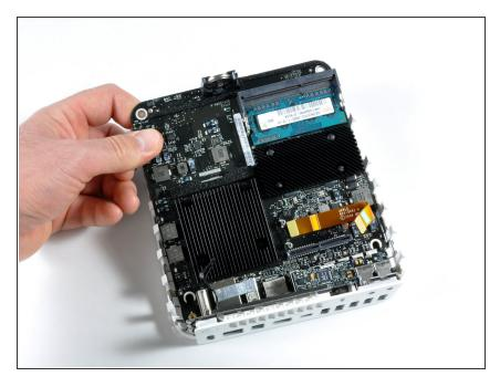
While slightly lifting the free end of the board pull it away from the port side of the mini, minding any edges that may get caught.
