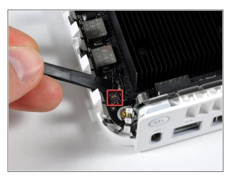
Use the flat end of a spudger to pry the power button cable connector up off the logic board.
