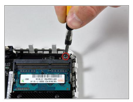
Remove the single T10 Torx lug next to the RAM sockets on the logic board.
