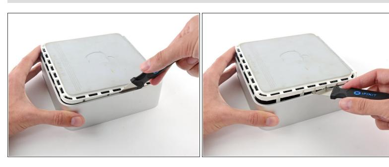
Keep working around the perimeter, freeing the clips along the final edge.
