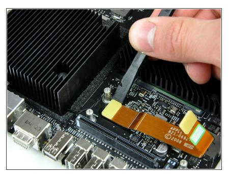
Use the flat end of a spudger to pry the AirPort/Bluetooth ribbon cable connector up off the logic board and set it aside.
