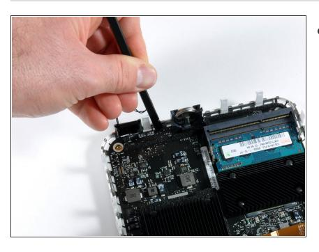
Use a spudger to lift the free end of the logic board off the bottom housing near the PRAM battery.
