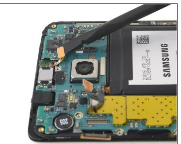
Use the flat end of a spudger to disconnect the front-facing camera ribbon cable.
