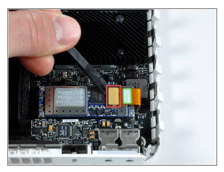
Use the flat end of a spudger to pry the AirPort/Bluetooth ribbon cable connector up off the combo card.
