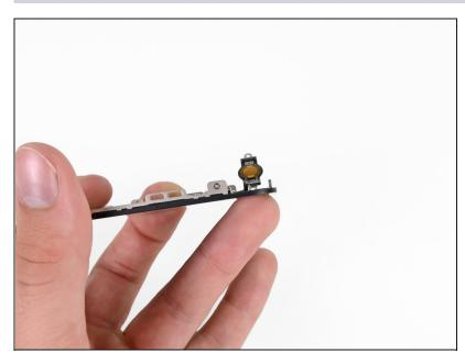
Gently press up on the center of the home button from the display side of the display assembly, to loosen the adhesive securing it to the assembly.
