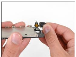
• Once the home button has started to separate from the display assembly, use the tip of a spudger to completely lift the button from the adhesive securing it.
