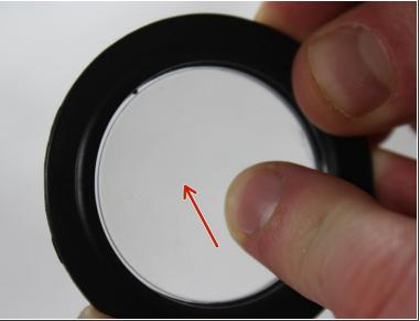
To get the actual lens out, you will need to push the lens from the outside in with a little force to break the lens out of it's case. To reassemble your device, follow these instructions in reverse order.
