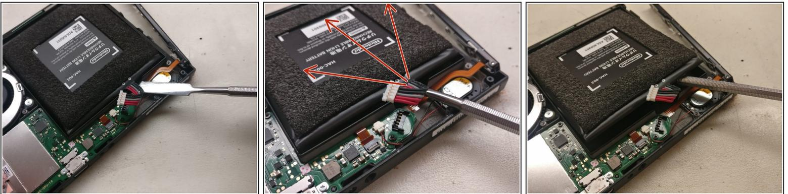
**⚠ Caution:** Lithium-ion batteries are fragile and can ignite if punctured or bent. Be careful when prying and do not use metal tools.
