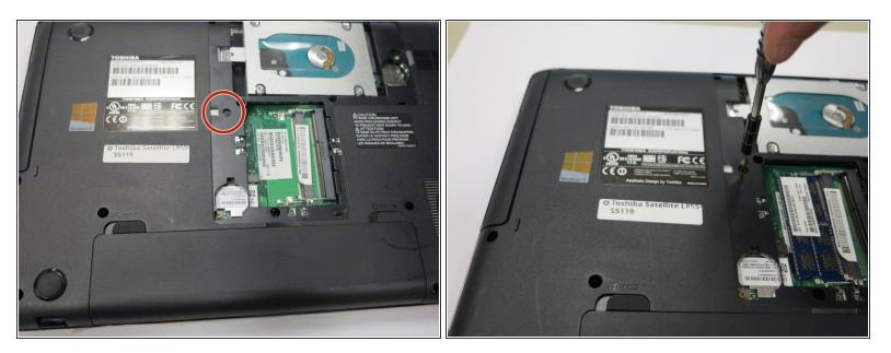
• Using a Phillips #0 screwdriver, remove the single 3mm screw.
