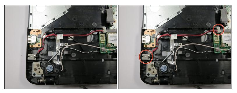
• Locate the DC power port. Note the 4-pin connector attaching the port to the motherboard.
