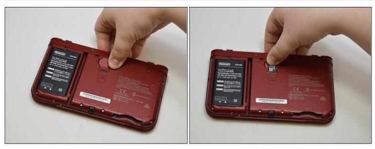
• Remove the microSD card by pushing it in, the card should automatically pop out.
