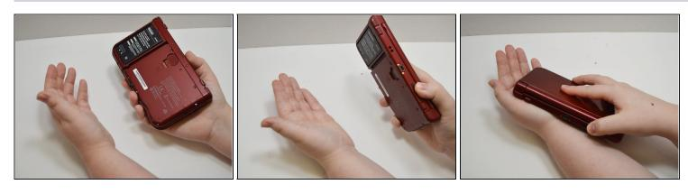
• To remove the battery, hold the device with the battery facing up in one hand, with a finger securely gripping the lid of the device, and gently flip the device over to your other hand. The battery should fall into your hand.
