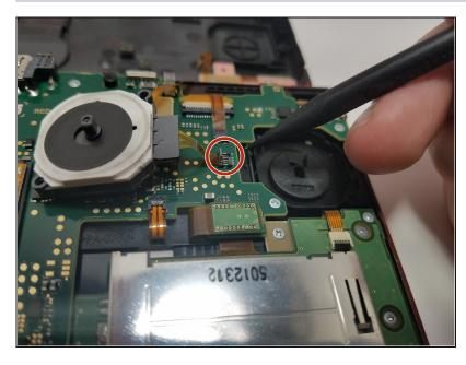
Using the tip of the spudger, gently lift off the lid of the ZIF connector to release the circle pad cable.
