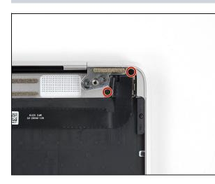
Remove two 2.5 mm Phillips #00 screws securing the USB-C port.
