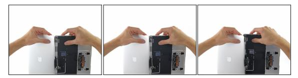
• Holding the display assembly with one hand and the upper case with the other, push them together slightly to move the hinges out of their recesses in the the upper case.
