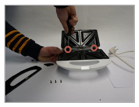
Unscrew two Phillips #0 screws of the top grill plate.
