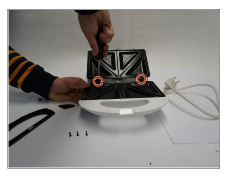
Unscrew two Phillips #0 screws of the lower grill plate.
