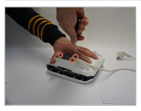
Unscrew three tri-wing screws of the plate on the bottom.
