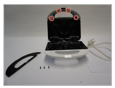
Unscrew four Phillips #0 screws of the black top plate on the inner side of the sandwich toaster.
