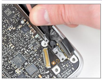
Use the tip of a spudger to gently peel the microphone off the adhesive securing it to the upper case.
