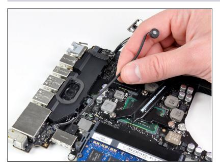
Remove the microphone from the logic board.
