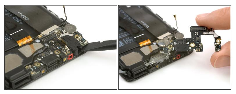
A Do not damage any components sitting on the charging board while removing it.
