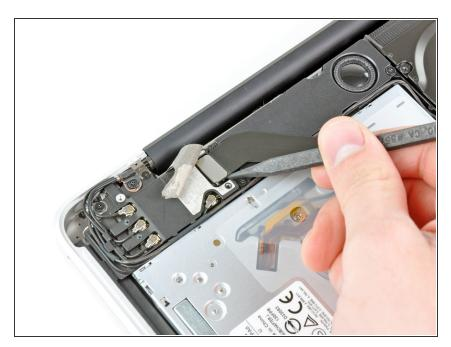
Use the tip of a spudger to lift the AirPort/Bluetooth connector off of its socket on the AirPort/Bluetooth board.
