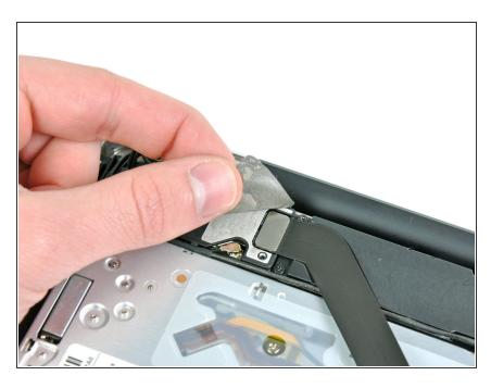
Peel back the piece of EMI tape covering the AirPort/Bluetooth cable connector above the optical drive.
