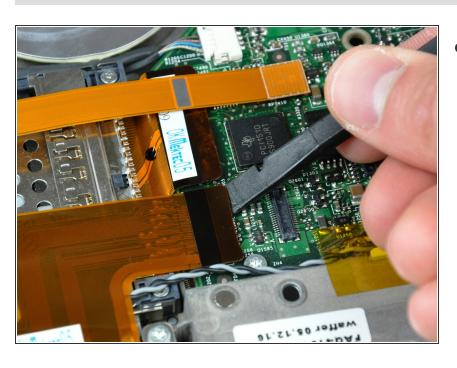
Use the flat end of a spudger to pry the hard drive ribbon cable connector up off the logic board.
