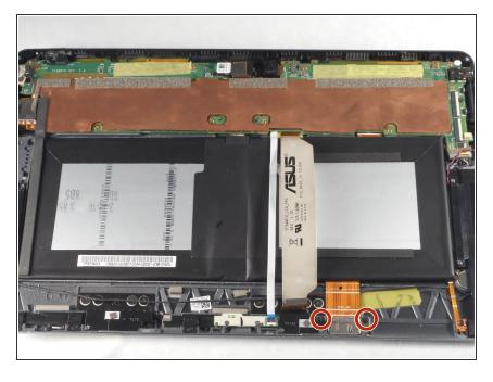
Remove the two 0.79mm screws from the charging port with the Phillips #00 screwdriver.
