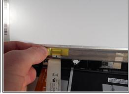
Remove the yellow tape that secures the digitizer and LCD screen ZIF connectors.
