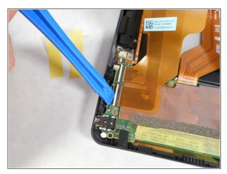
After removing the yellow tape, use a plastic opening tool to lift the two digitizer ZIF connector tabs; pull the ribbon cable free.
