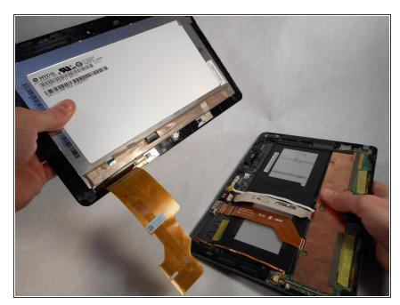
• Lift the screen upwards to remove.
