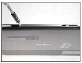
Rotate the device 180°, and use a PH000 screwdriver to remove the two 1.59 mm screws at the bottom.
