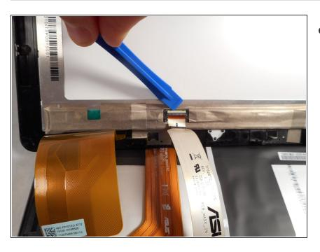
Use a plastic opening too to lift the LCD screen ZIF connector; pull the ribbon cable free.
