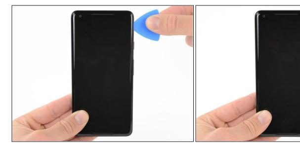
Slide the opening pick down the right side of the phone to separate the display adhesive.
