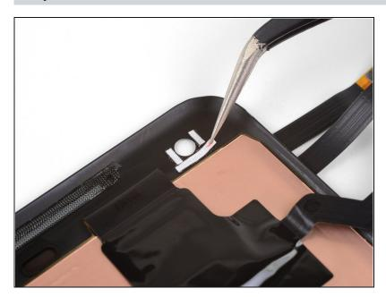
Peel the white backing off of all three adhesive strips.
