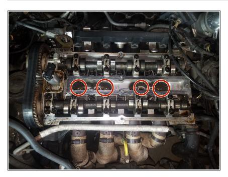
Remove the four spark plugs using a 5/8" spark plug socket
