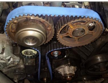
Starting on the crankshaft sprocket, slip the belt around it, working clockwise around the tensioner pulley, intake sprocket, exhaust sprocket, then idler pulley, all while keeping the belt under tension
