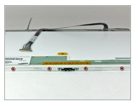
Remove the four black Phillips screws along the top edge of the display.
