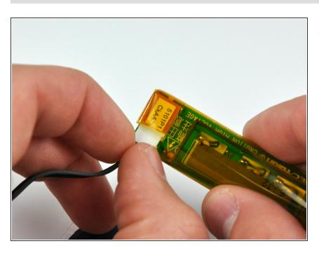
Disconnect the inverter cable by pulling its connector away from the socket on the inverter board.
