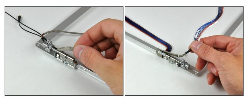
De-route the inverter and display data cables from the clutch hinges and set them aside.
