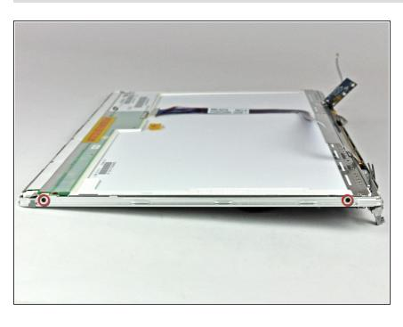
Remove the two black Phillips screws from either side of the display (four screws total).
