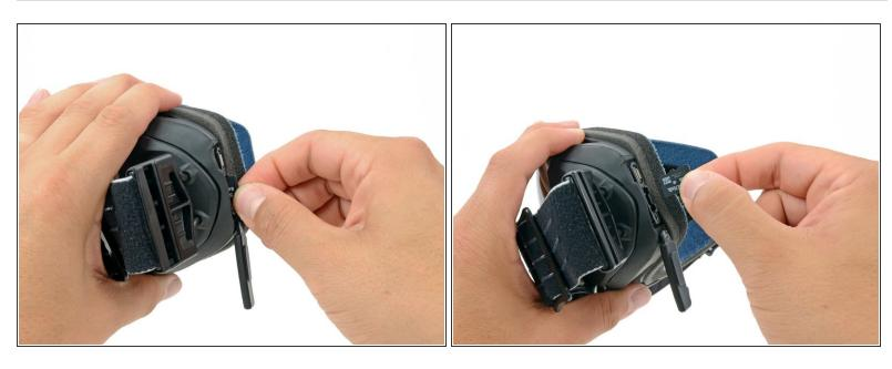
Pull the memory card straight out of its slot.
