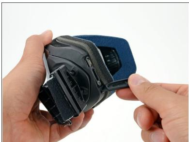
Peel the rubber cover for the memory card and USB port away from the goggles.
