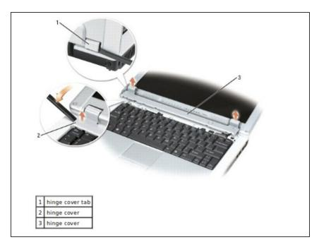
Use a plastic flat screwdriver to slide the hinge caps away from the computer.
