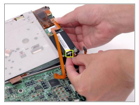
• Lift of the right side of the optical drive and disconnect the modem cable.
