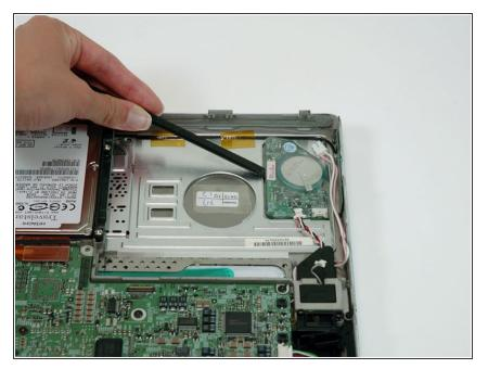
Use a spudger to pry the PRAM battery out of its housing on the upper case. Make sure not to bend the PRAM battery too much while prying it out.
