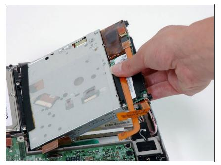
• Lift the optical drive up and out of the computer.
