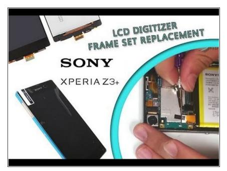
In this guide I will present you how to replace cracked display in your Xperia Z3 Plus (Z4) smarpthone.
