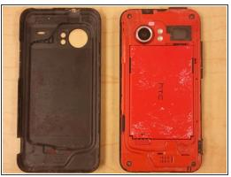
Pry off back plastic, starting at the gap provided at the bottom of the phone. A spudger can be used to make this easier.
