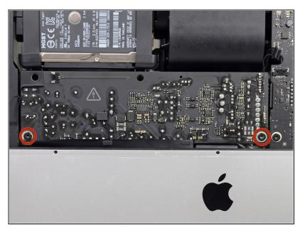
Remove the two 7.2 mm T10 screws securing the power supply to the rear enclosure.
