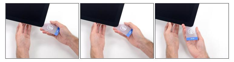
• Insert a second plastic card into the gap between the display and frame located at the top left corner of the iMac.
