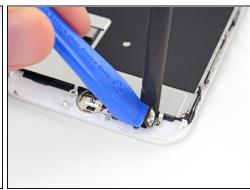
Use an opening tool to pry under the left edge of the home button cable connector to disconnect it from its socket.
