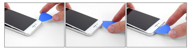
• Slide an opening pick underneath the display around the top left corner and along the top edge of the phone to loosen the last of the adhesive.
