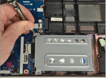
• Use a #0 Phillips screwdriver to remove the two 4mm screws securing the hard drive carriage in place.
