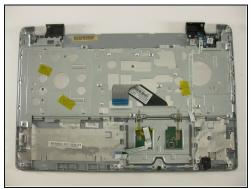
• Once all three ribbon cables are disconnected, lift off the top cover with the keyboard and touchpad.
