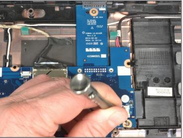
Use a #0 Phillips screwdriver to remove the two pictured 4 mm screws.
