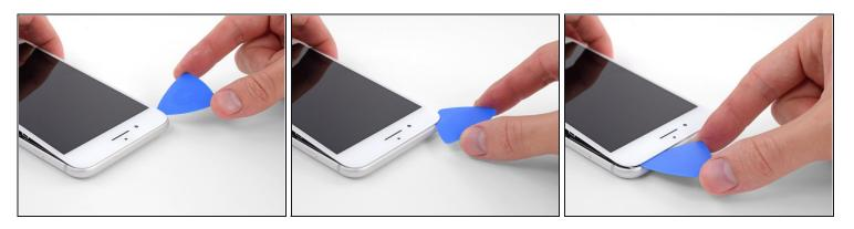
• Slide an opening pick underneath the display along the top edge of the phone to loosen the last of the adhesive.
