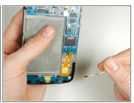
Remove the white antenna interconnect cable that attaches the motherboard to the bottom righthand corner of phone by pulling on it gently.
