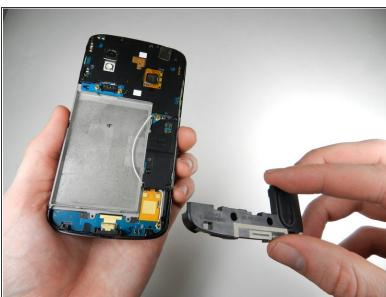
Gently pry the speaker up and away from the back of the phone using a plastic opening tool, and lift it out of the phone.
