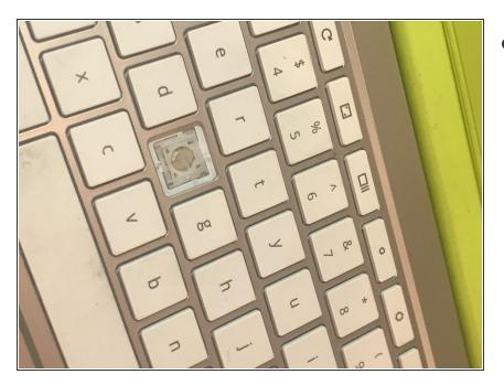
Take a flathead screw driver and place it right under the key. Very gently pry it up. If it doesn't come off right away, try and loosen it by using the flathead on all four sides and wiggle it.
