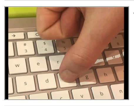
Once the key is off, all you have to do to put a new key on is center it exactly how the original one was, and push down.
