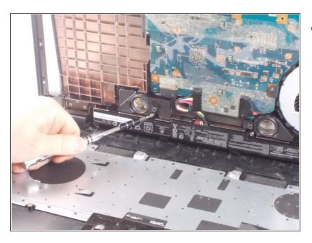
Unscrew the two 8mm screws attached to the battery
