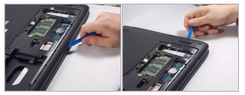
• Use the opening tool to pry the back of the laptop case from the top
