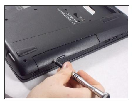
Begin by putting the needle into the hole in the disk tray.
