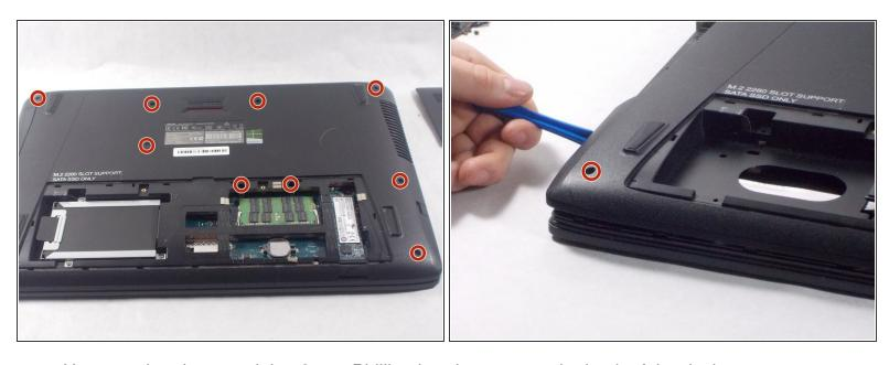
Unscrew the nine remaining 8 mm Phillips-head screws on the back of the device.
