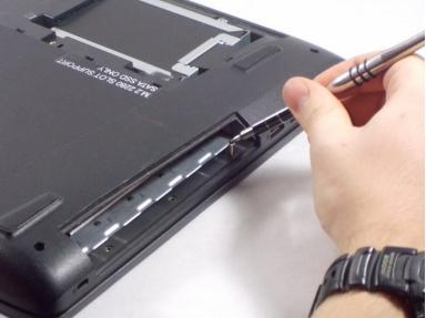
Remove the 3 small screws located underneath the disk drive.
