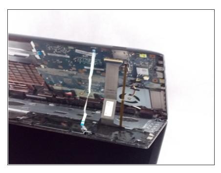
Disconnect the 3 cables connecting the motherboard to the keyboard.
