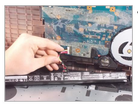
Disconnect the bundled cable connector and remove the battery.
