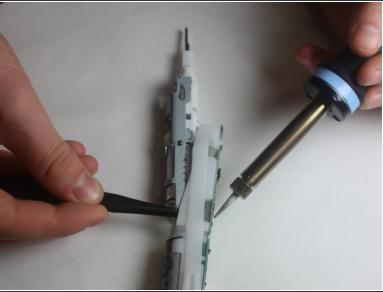
Desolder the motor terminals from the motherboard and remove the motor assembly.
