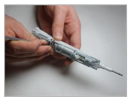
Remove the spring from the housing using a nylon spudger.
