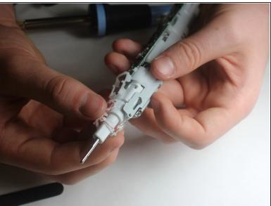
Use a pair of tweezers to remove the plastic housing and the LED from the device.
