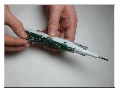
Remove the indicator light lenses from the motherboard using your fingers or a spudger.
