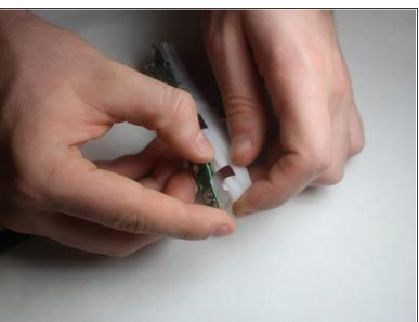
All points of contact between the mother board and the other components should now be desoldered. Remove the motherboard by gently pushing up on it, pulling it out of the plastic tabs that secure it to the housing.
