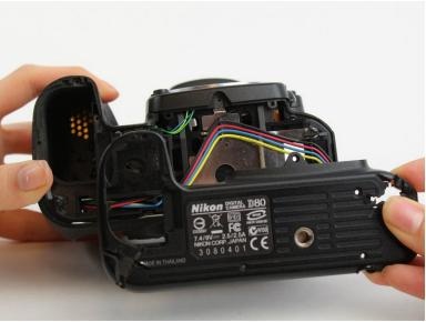
• Use the plastic opening tool to remove the bottom cover.
