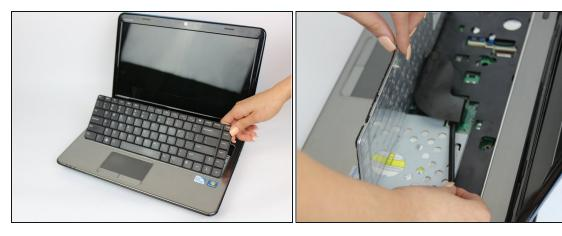
• Carefully tip the keyboard upwards and pull it slightly away from the body of the laptop.
