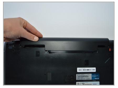
• Gently slide the battery out while still holding the left unlock switch.
