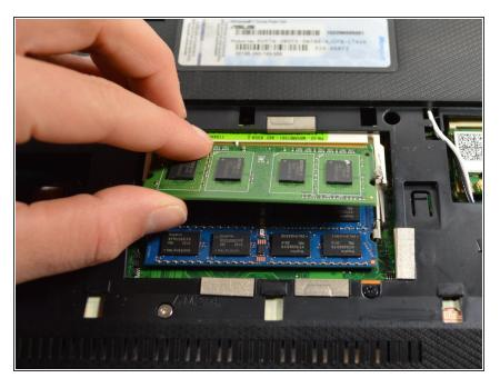
Remove the RAM by lifting up with your fingers and sliding it out towards you.
