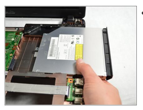
Slide the optical drive out. It should easily come out.
