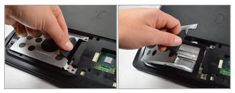
• Remove the hard drive by sliding it to the left and lifting up.
